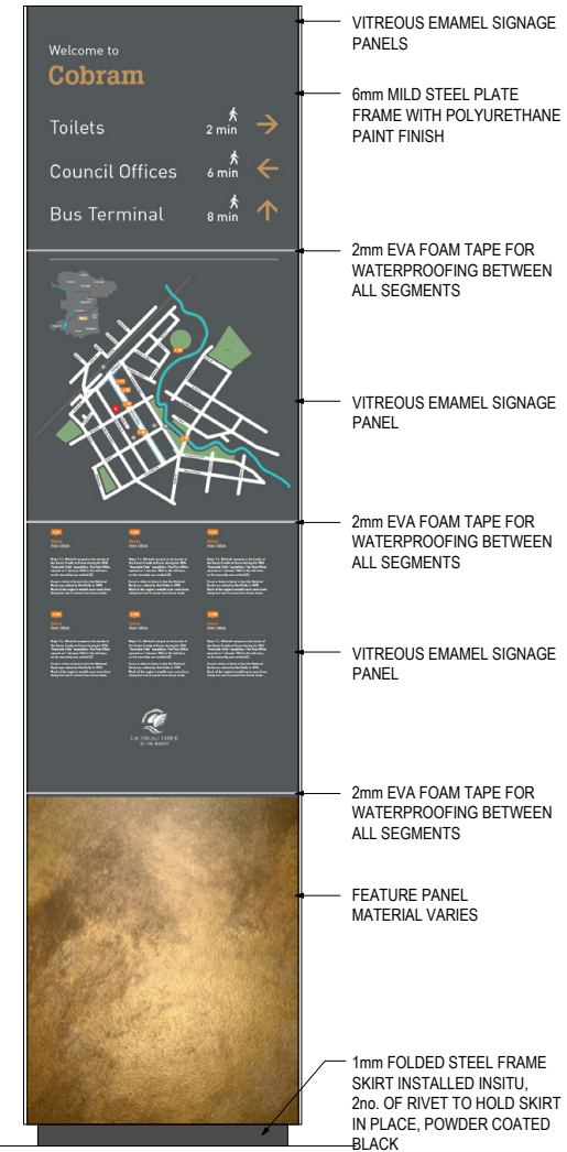
2 TYPICAL PLINTH FRONT VIEW Scale: 1:10
