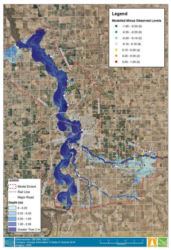
FIGURE 5-9 HYDRAULIC MODEL CALIBRATION PLOT - SEPTEMBER 2010
