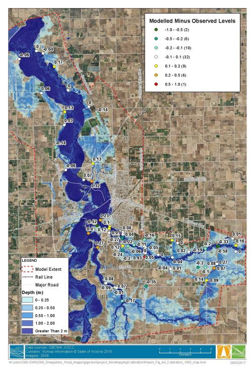
FIGURE 5-14 HYDRAULIC MODEL CALIBRATION PLOT - OCTOBER 1993 EVENT
