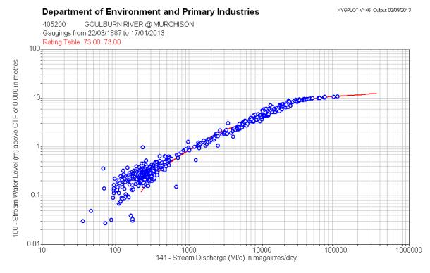
FIGURE 4-2 MURCHISON CURRENT RATING CURVE AND GAUGINGS (SOURCE: DELWP)
