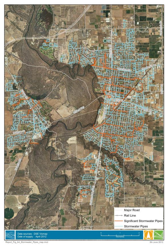
FIGURE 3-6 SHEPPARTON-MOOROOPNA STORMWATER PIPE SYSTEM
