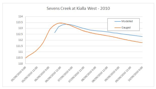
FIGURE 5-8 COMPARISON BETWEEN MODELLED AND GAUGED WATER LEVELS FOR THE SEVEN CREEKS AT KIALLA WEST DURING THE SEPTEMBER 2010 EVENT
