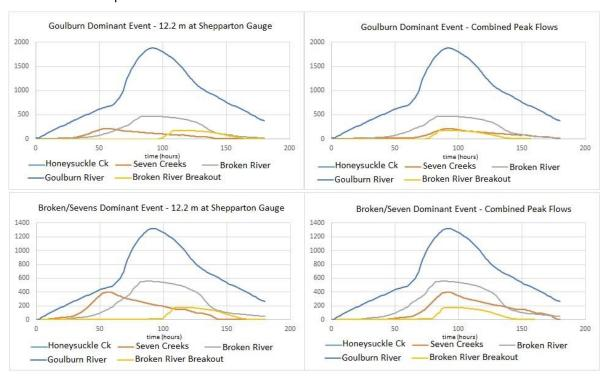
FIGURE 6-1 INFLOW HYDROGRAPHS FOR SENSITIVITY ANALYSIS OF TRIBUTARY TIMING
