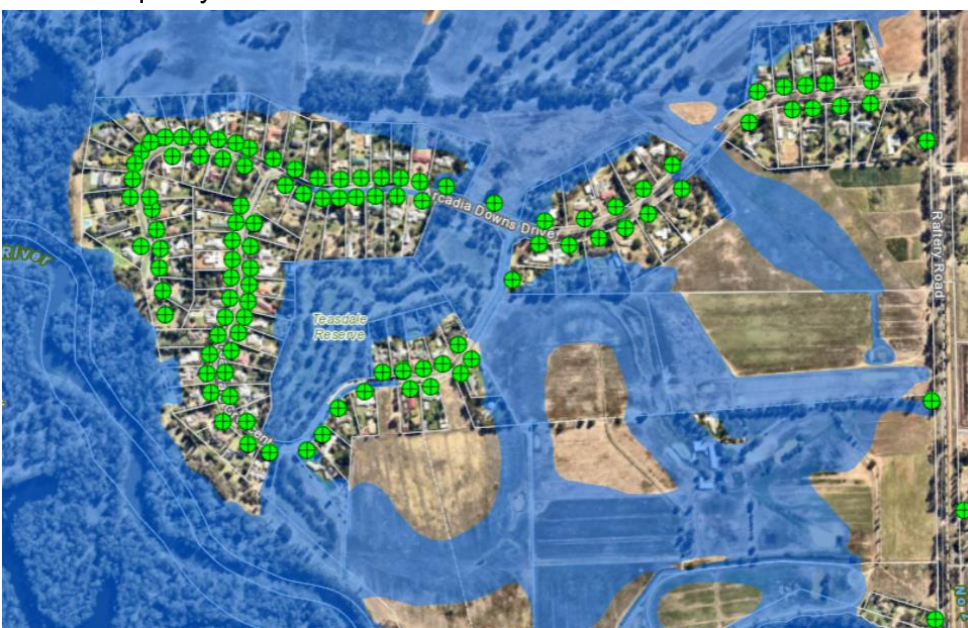
Image 3: Planning and development controls in areas liable to flooding for the Arcadia Downs Estate minimizing flood impacts to dwellings. Knowledge of flood overlays are used to ensure septic tank systems are not installed in land subject to inundation or flooding.
