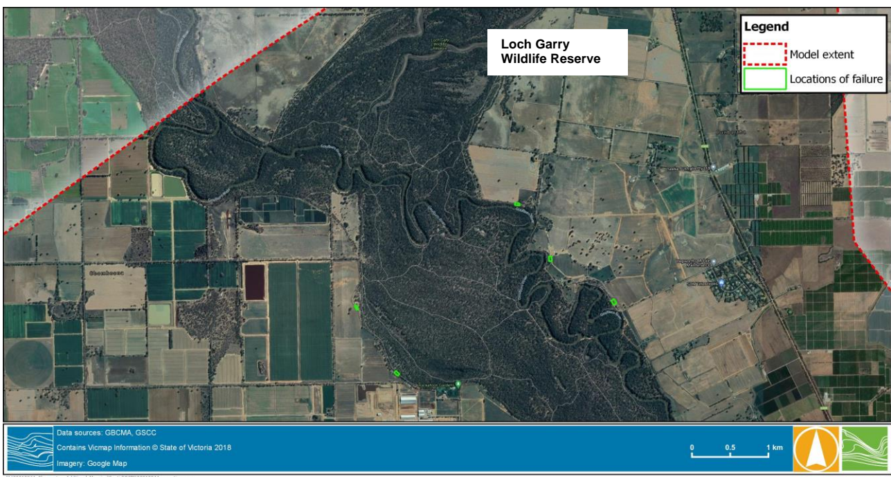
FIGURE 8-1 LOCATIONS OF LEVEE FAILURES
