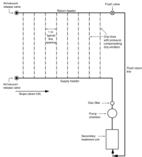
Image 20: Diagram of pressurized sub-surface drip irrigation
