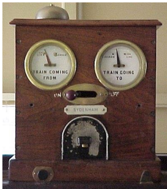
Old Double Line Block safeworking instrument similar to those still in use between Craigieburn and Seymour
