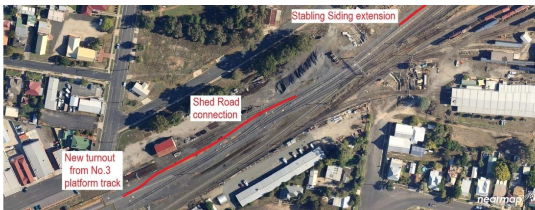
Aerial photograph of Seymour station and yard (Down end) showing proposed alterations
