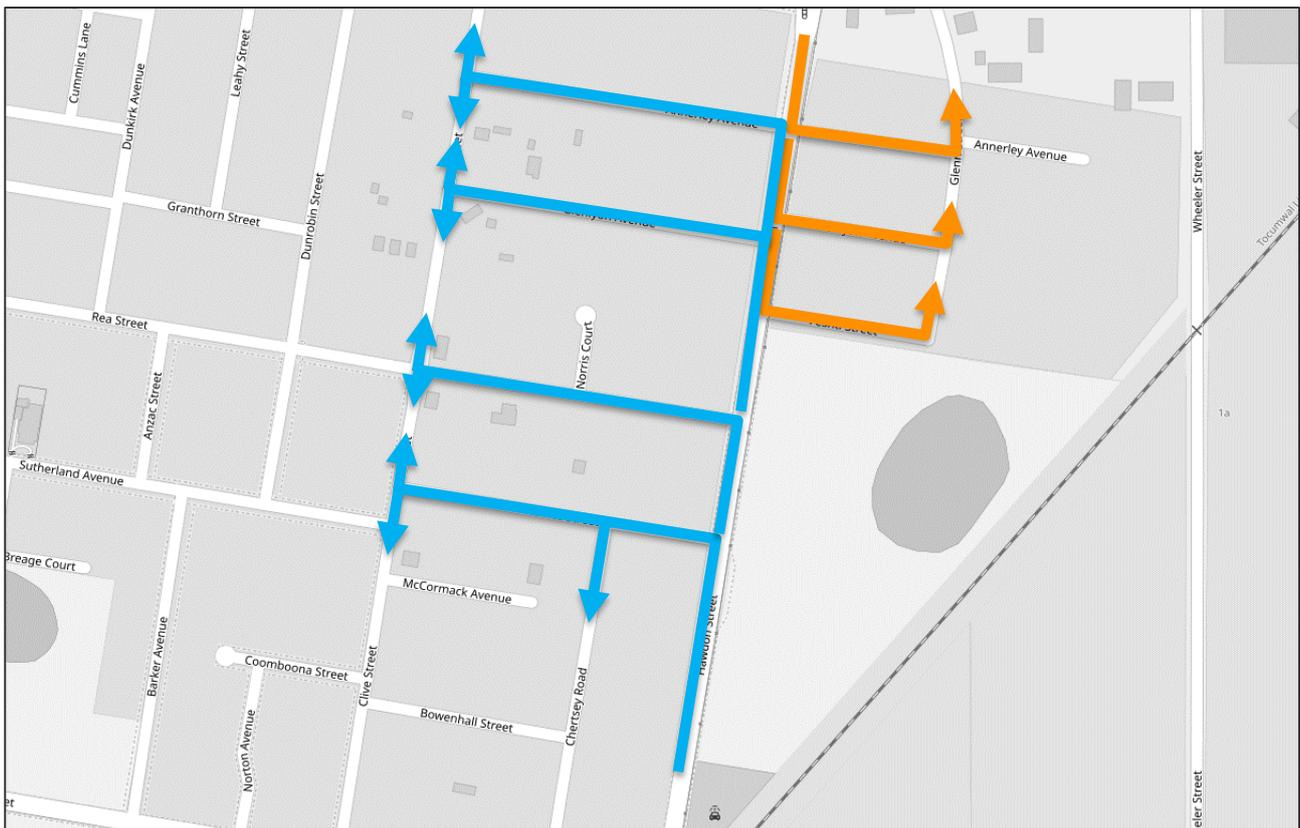
Coupled with restrictions on right-turn movements at key side-streets (discussed within Section 9.1), this will greatly assist with minimising the impacts of turning movements to and from Hawdon Street.
