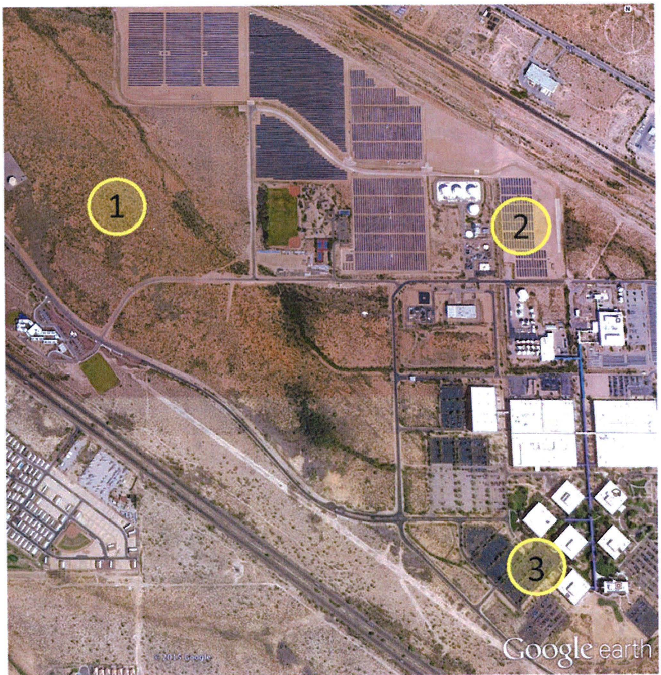
Figure 4: Experimental sites. Monitoring a (1) natural semiarid desert ecosystem, (2) solar (PV) photovoltaic installation, and (3) an “urban” parking lot – the typical source of urban heat islanding – within a 1 km 2 area enabled relative control for the incoming solar energy, allowing us to quantify variation in the localized temperature of these three environments over a year-long time period.
