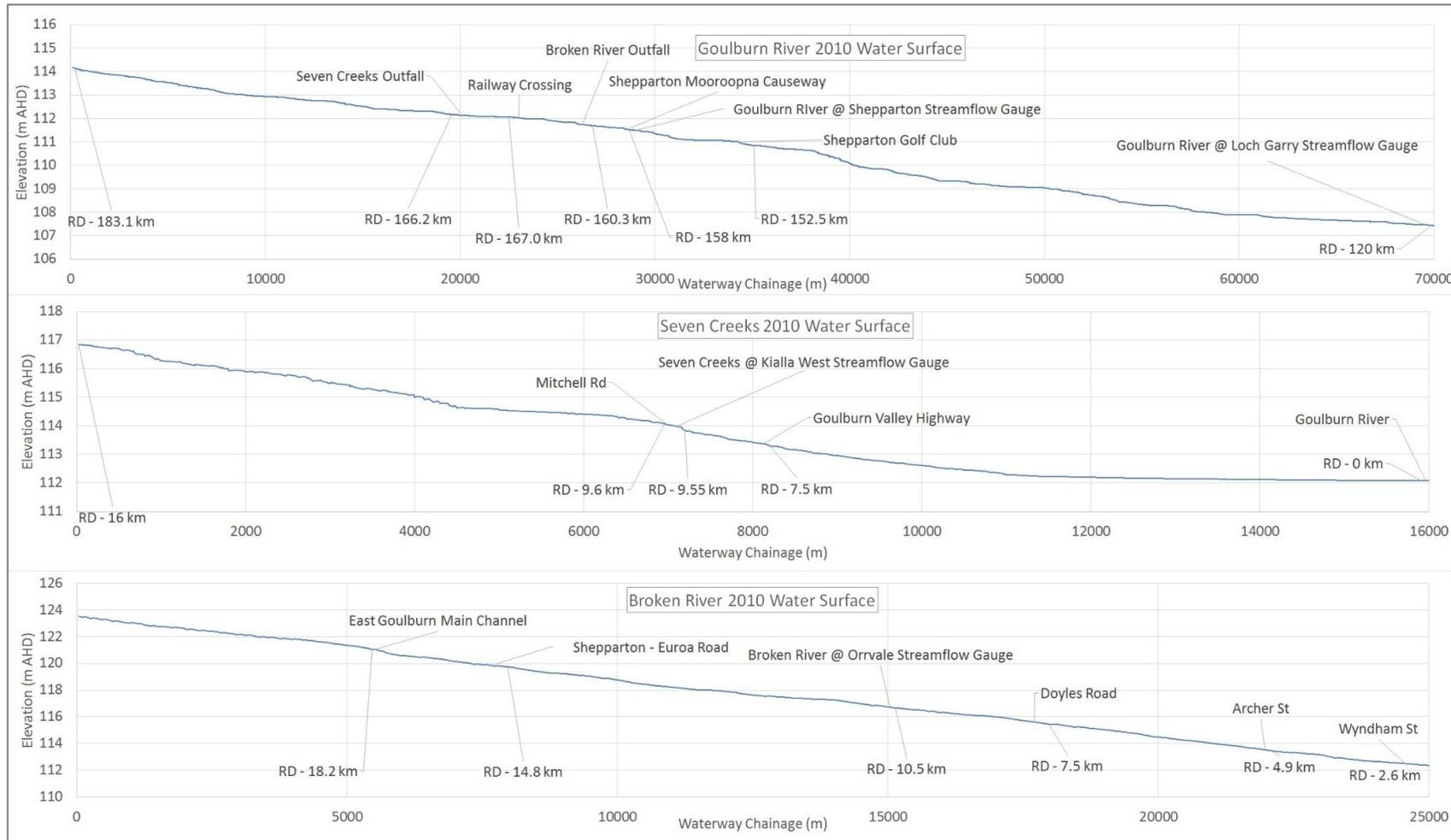
**FIGURE 5-11 SEPTEMBER 2010 – WATER SURFACE PROFILES**
