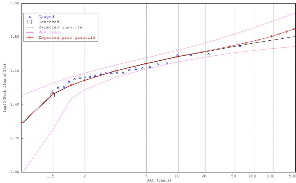
**FIGURE 4-4 GEV DISTRIBUTION FITTED TO ANNUAL SERIES FOR BROKEN RIVER @ ORRVALE (404222)**
