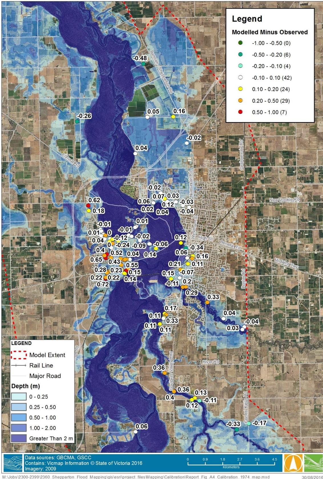
**FIGURE 5-18 HYDRAULIC MODEL VALIDATION PLOT – MAY 1974 EVENT**
