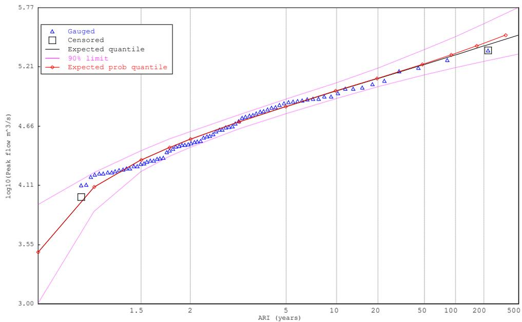
**FIGURE 4-11 GEV DISTRIBUTION FITTED TO ANNUAL SERIES FOR GOULBURN RIVER @ SHEPPARTON (405204)**
