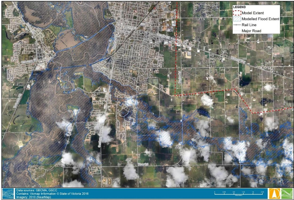
**FIGURE 5-10 SEPTEMBER 2010 MODELLED FLOOD EXTENT AERIAL IMAGERY VALIDATION (SOURCE: NEARMAP)**
