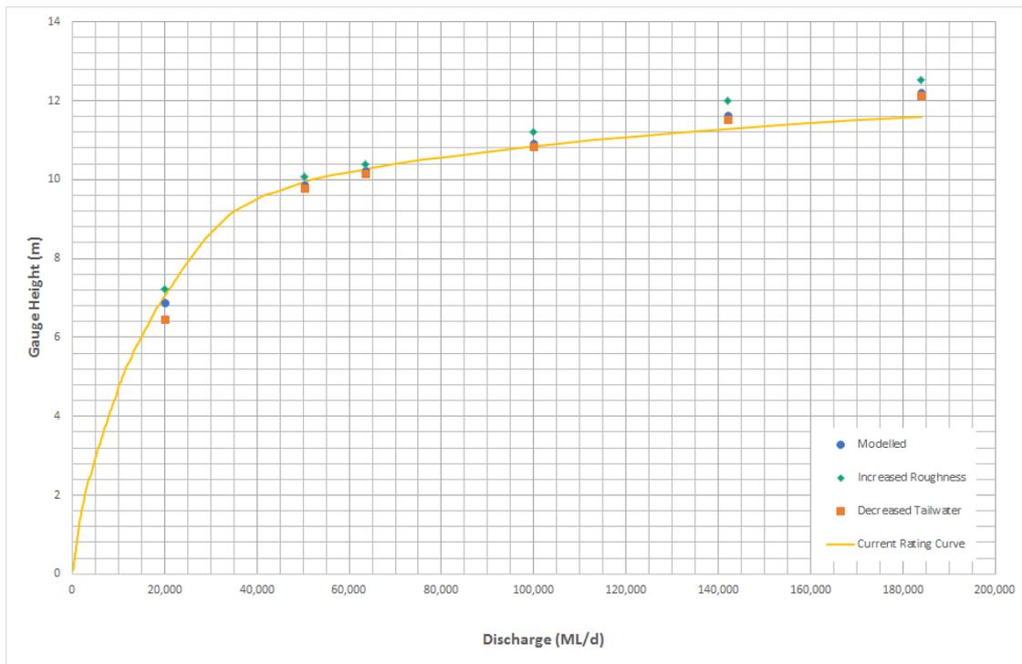
**FIGURE 4-3 MURCHISON CALIBRATION AND SENSITIVITY RESULTS**
