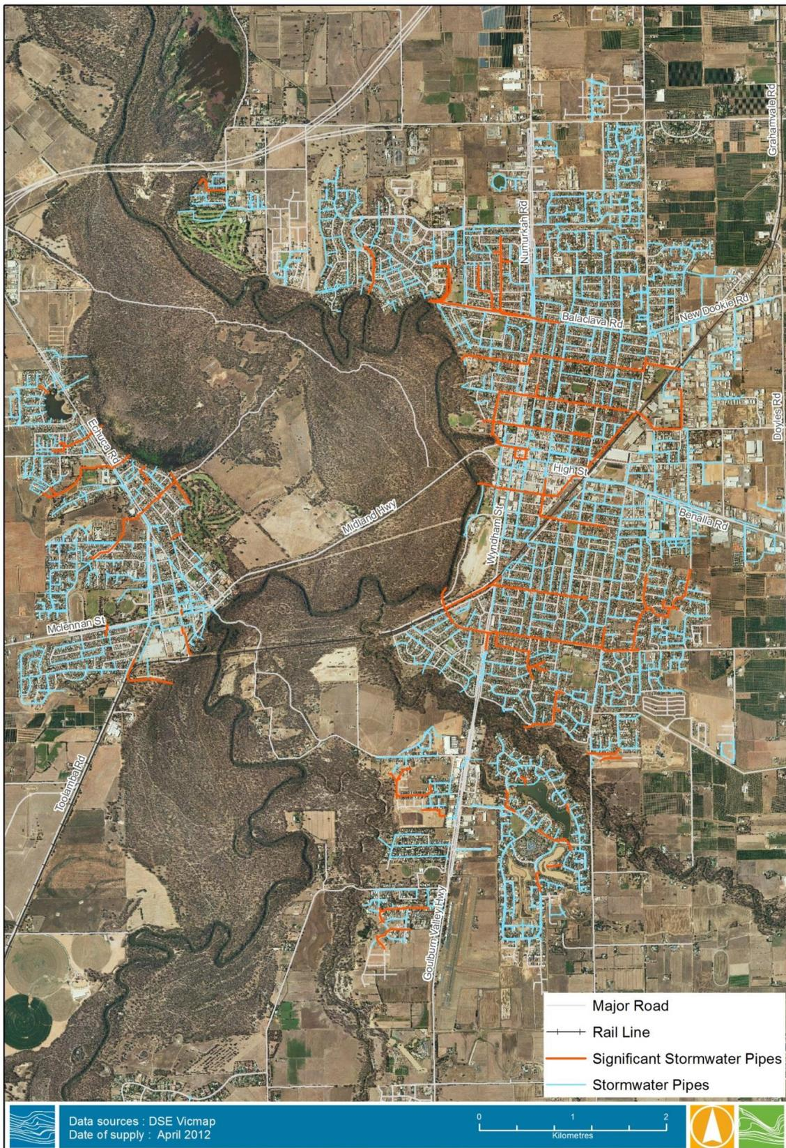
**FIGURE 3-6 SHEPPARTON-MOOROOPNA STORMWATER PIPE SYSTEM**
