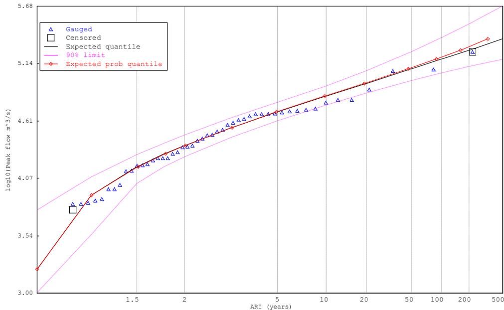
**FIGURE 4-8 GEV DISTRIBUTION FITTED TO ANNUAL SERIES FOR GOULBURN RIVER @ MURCHISON (405200), REVISED RATING CURVE DATA, POST-BIG EILDON RECORD PLUS 1916**
