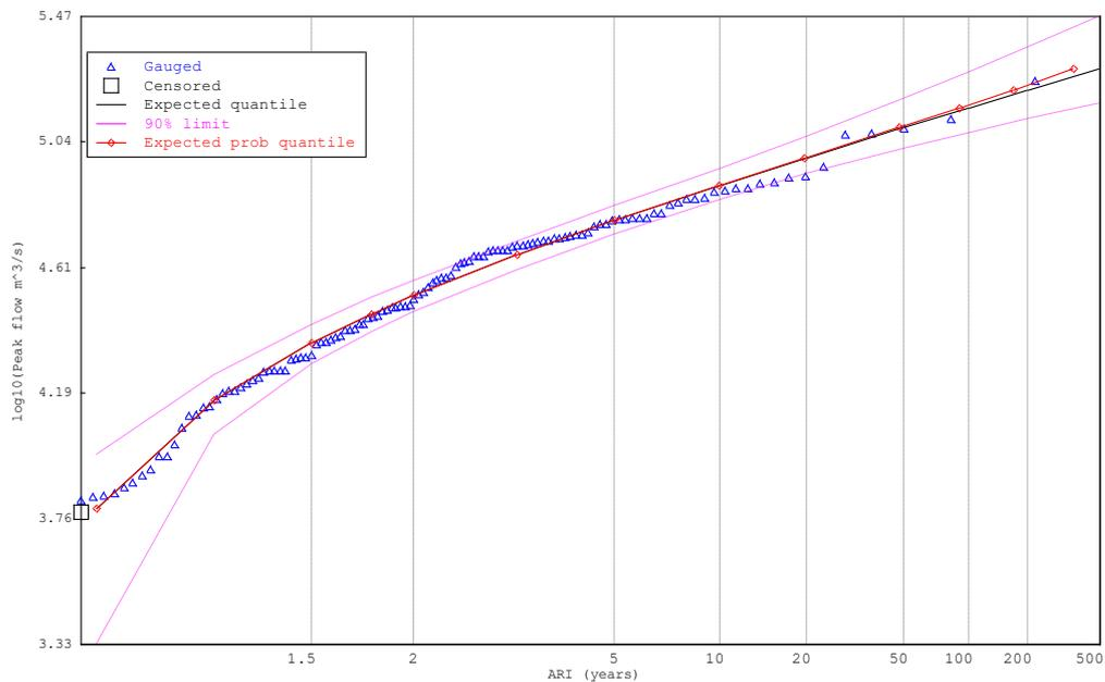
**FIGURE 4-9 GEV DISTRIBUTION FITTED TO ANNUAL SERIES FOR GOULBURN RIVER @ MURCHISON (405200), REVISED RATING CURVE DATA, ENTIRE RECORD**
