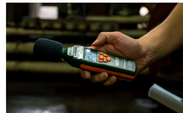
Checking sound levels
